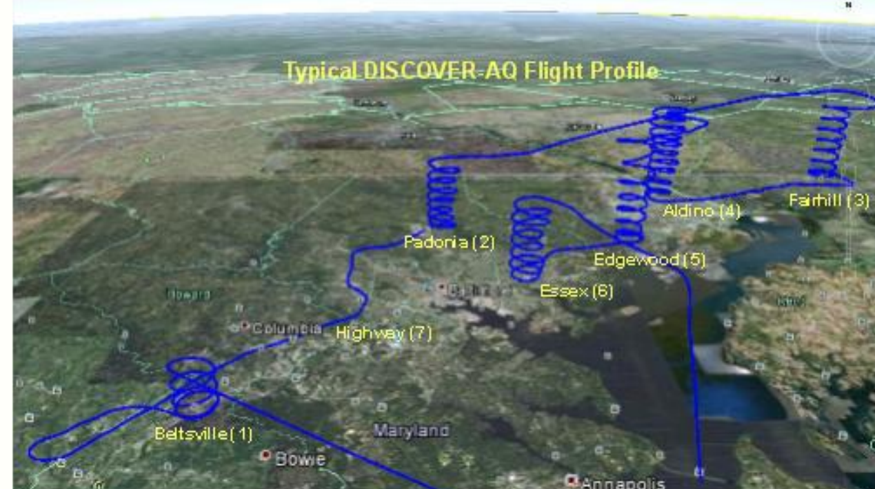
Typical flight track showing spiral points over ground sites. The flight track was normally repeated four times during each flight day.
